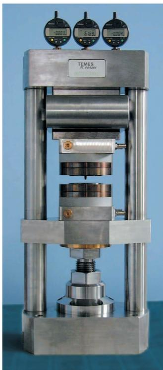
In those cases in which a creep of the gasket could lead to an unloading of the flanged joint, gasket factors from creep relaxation tests are of interest. Influencing parameters can be stiffness, temperature, temperature changes, time etc. It is necessary to perform a lot of tests and most of them are of long term nature.
