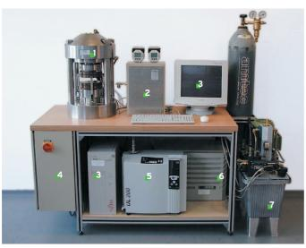
every relevant gasket factor, e.g. testing according ASTM and PVRC methods, EN 13555 or DIN 28090. Thus it is possible to determine every necessary gasket factor for the selection of the gasket and for an analysis of the joint.
