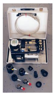
If the demands are stringent, e.g. regarding stuffing boxes in systems with dangerous or poisonous media, an explicit control of successful tightening may be necessary, additionally to the use of hydraulic tensioners.
