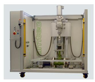
In addition to the test rigs to determine all relevant packing material characteristics, **amtec** developed a testing equipment for valves, **TEMES** *valve.teq*,
