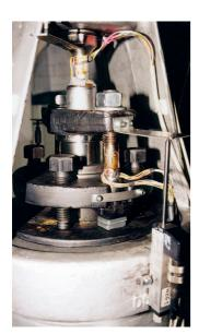
Regarding safety relevant valves, it is often necessary to prove function which means in most cases a check of stem friction forces during planned outages. On the basis of monitoring results, the relevant parameters can be evaluated and
