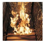
accepted applications/qualification tests. One example is a test rig for fire safe tests. **amtec** developed this test rig to complete its scope of services and products.
