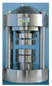
and heating platens can be exchanged, but also the gasket platens for tests of different gasket designs (e.g. gaskets for floating type or metalto-metal type joints).
